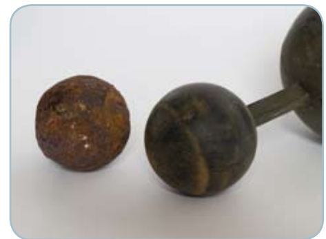
A year after installation, this is the condition of a metal ball of the type normally used in competitor flushing valves (left) and the rubber ball used in the Zenit FLX.
